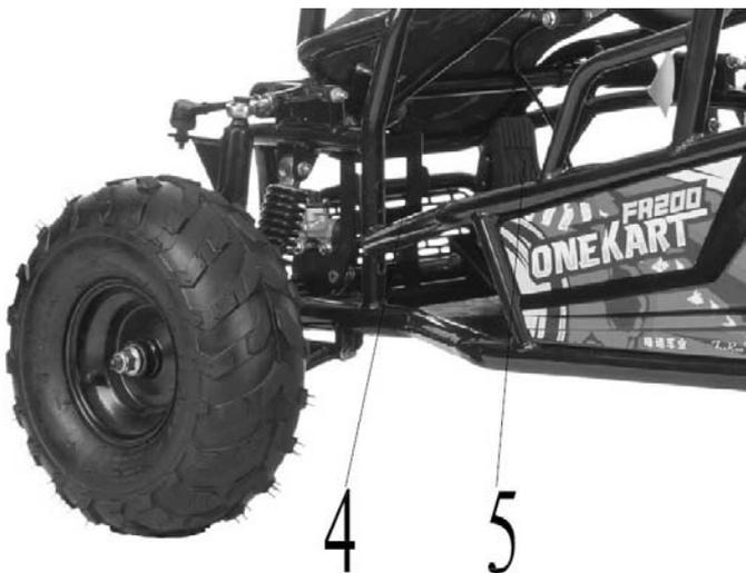
**Brake Pedal (4):** Depressing the brake pedal will stop the Go Kart. Note: Always check brakes before operation .
