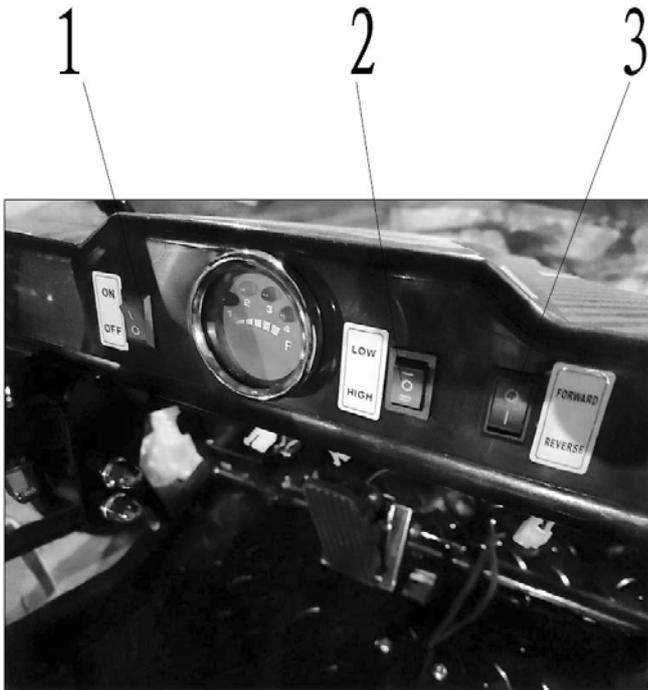
**Main Switch (1):** When the main switch is placed in the (ON) position the motor can runs.
