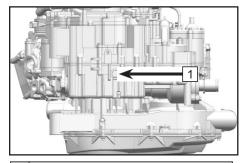
1 Drain bolt, Engine oil
