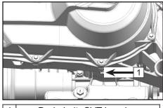
Drain bolt, CVT housing
