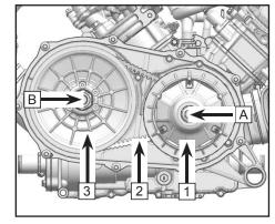
The secondary clutch (3) is mounted to the input shaft of the transmission (B) and serves two functions; As a "slave" pulley to the primary clutch, and to provide a torque sensing element that shifts drive ratios. The drive belt (2) is a heavy duty V-belt that connects the engine and transmission clutch pulleys.
