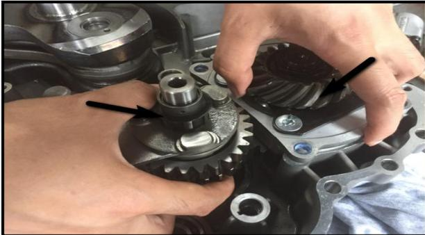
c. Lift the shift forks (and not the shift fork shaft) as required to install the shift fork pins into the shift drum grooves while sliding the shift drum into position. Make sure the shift fork shaft and shift drum are both bottomed in the case half.
